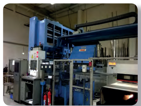
Laser MAZAK STX48 MKIII 4000 W + Robot LD48
