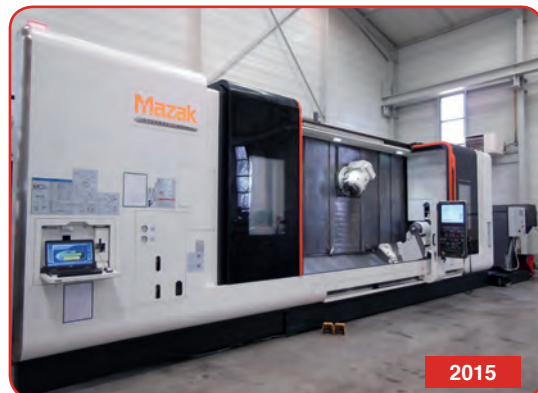
MAZAK INTEGREX E670h II CNC MAZATROL MATRIX 2 5 axes - EP 4000
