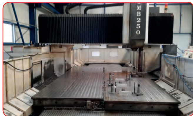
SMTCL GMB 250 CNC FANUC 18i MB X=5200 Y=3200 Z=1000 mm
