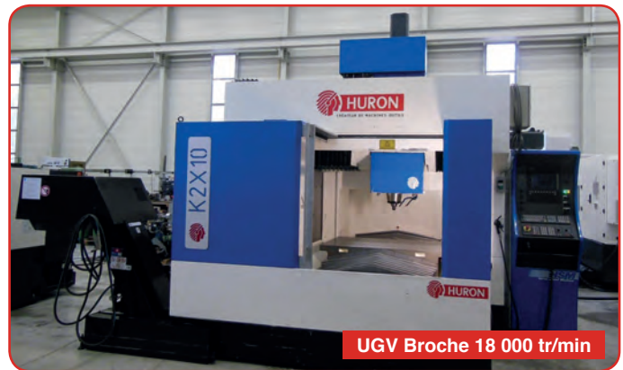
HURON K2X10 CNC SIEMENS 840D POWERLINE X=1000 Y=800 Z=500 mm
