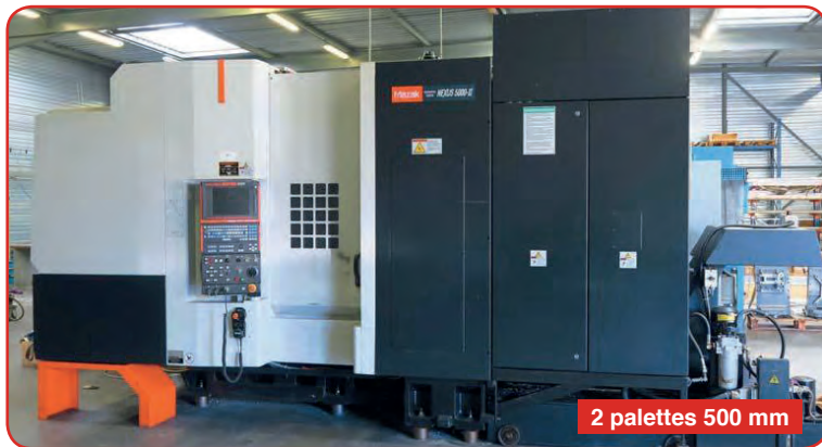
MAZAK NEXUS 5000 - II CNC MAZATROL NEXUS X=730 Y=730 Z=740 mm
