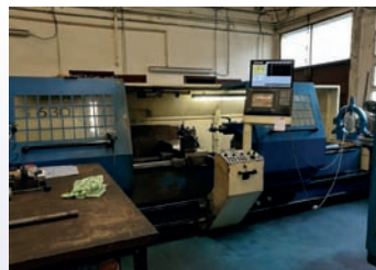
Tour CNC VOJUS TURNTEC 63 x 3000 MMh Dia 630 x 3000 mm Lunette Siemens 840 D Shop Turn
