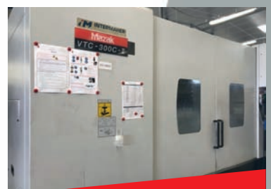
Centre d'usinage vertical MAZAK VTC 300C II - CNC MAZATROL 640 M Table 2000 x 760 mm Courses 1740 x 760 x 660 mm
