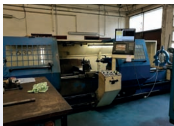
Tour CNC VOJUS TURNTEC 63 x 3000 MMh Dia 630 x 3000 mm Lunette Siemens 840 D Shop Turn
