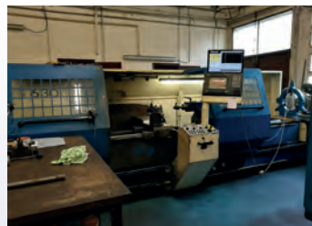
Tour CNC VOJUS TURNTEC 63 x 3000 MMhh Dia 630 x 3000 mm Lunette Siemens 840 D Shop Turn
