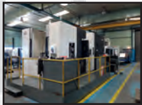
Centre horizontal OKUMA MA-600H de 2014 BT 50 Big + 2 palettes 630 x 630 X 1000 x Y 900 x Z 1000
