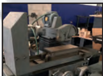
Rectifieuse plane SIT RA HLT Long. 450 x larg. 160 mm
