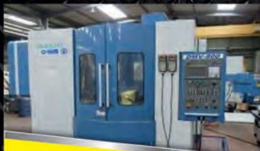
Centre DHALI DMV 800 Roto palette FANUC 800 x 560 x 560
