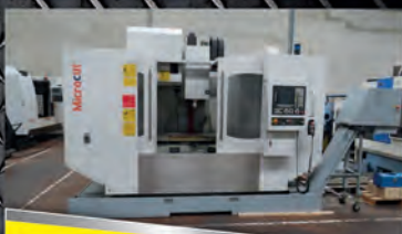
Centre MICRO CUT MM1000 CNC FAGOR 8055 1000 x 580 x 550
