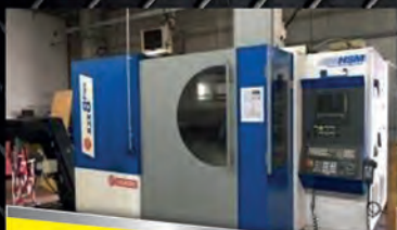
Centre HURON K2X8F - 5 axes CNC SIEMENS 840 D Crs 850 x 700 x 450
