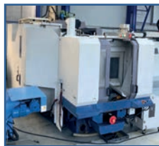
CU horizontal Mori Seiki SH 5000/40 Double palettisation 500 x 500 mm X 800 x Y 700 x Z 700 mm - B continu 360° Rapides 50 m/min - Broche 20.000 tr/min 22 kW
