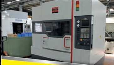
Centre QUASER MV 184P - 2011 Fanuc 18iMB M Guide-ST - 1200 x 600 Palpeur - Arrosage centre - Convoyeur
