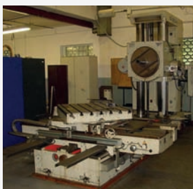
Aléuseuse SCHARMANN type FB100A Ø broche 100 mm - cône SA50 X = 2500 mm Y = 1200 mm Z = 1200 mm Plateau Ø 650 - visu 3 axes
