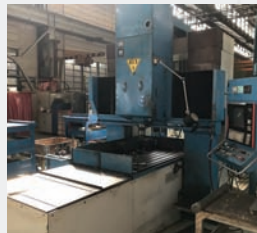
Pointeuse verticale CNC WMW MIKROMAT Type BKOZ 900x1400/5NC Courses X 1120 mm - Y 710 mm Z 315 mm CN NUM 1060 Table 1400 x 900 mm
