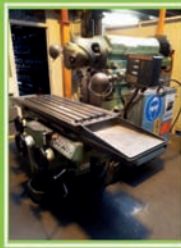
AV Fraiseuse HURON NU3 Courses : 900 x 700 x 500 mm I & A DUFOUR + 33 (0)3 25 43 85 60 commercial@ia-dufour.fr www.ia-dufour.fr
