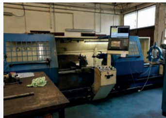
Tour CNC VOJUS TURNTEC 63 x 3000 MMhh Dia 630 x 3000 mm Lunette Siemens 840 D Shop Turn
