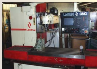
Fraiseuse LAGUN FBF 1200 100 x 600 x 600 HEIDENHAIN TNC 355
