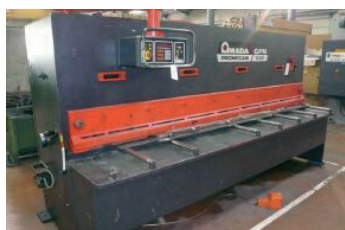
Cisaille AMADA type GPN 630 Cap. 3 000 x 6 mm
