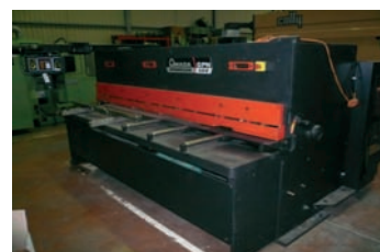
Cisaille AMADA type GPN 425 Cap. 2 500 x 4 mm
