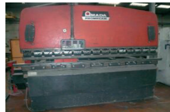
Presse plieuse AMADA type ITS CN 2 axes - Cap. 125T x 3 000
