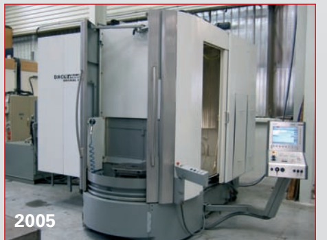
DMG DMC 70 Evolution SIEMENS 840 D 5 axes - X=750 Y=600 Z=520 - 2 palettes - 32 outils 18 000 t/min
