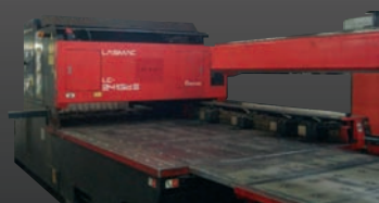
Laser AMADA LASERMAR LC 2415 alpha III 4 Kw - 2 520 x 1 550 mm 2004
