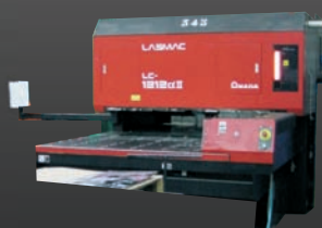
Laser AMADA LASERMAR LC 1212 alpha II 3 Kw - 1 250 x 1 250 mm 1999
