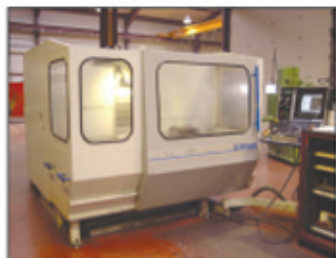
MIKRON WF 72C X 900 mm - Y 630 mm - Z 500 CNC HEIDENHAIN TNC 425 - Magasin 22 Outils - Tête escamotable
