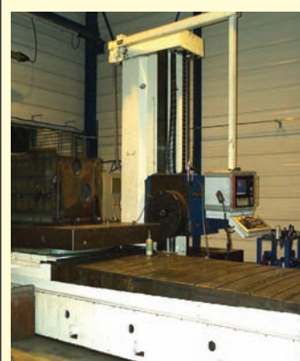
PEGARD AF 110 (1975/2000), X = 3.500, Y = 2.000, Z = 1.500, W = 800 mm, axe B 360.000 positions 2.400 x 1.800 mm, CN NUM 1060 5 axes.
