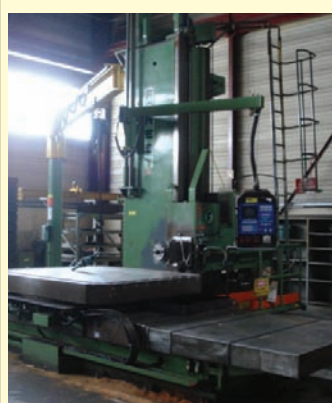
FOREST LINE P 2000 (1978/1986) X = 3.200, Y = 2.500, Z = 800, W = 1.250 mm, table 2.000 x 2.300 mm, B 360.000 positions, charge 15 T, tête de fraisage universelle CORREA, CN NUM 760 5 axes.
