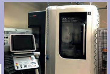
CUV 5 axes DMG DMU 40 EVO
