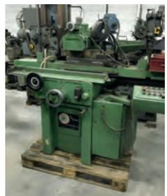
AV Rectifieuse plane MONOPRECIS - Type RHE 200
