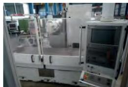
AV Fraiseuse CNC HURON PUXR 771 - Heidenhain TNC 426 - Course axes X 1485, Y 753, Z 991 mm
