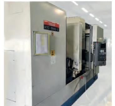
AV Centre vertical MAZAK VTC 300C
