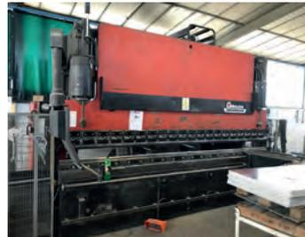
AV Presse plieuse AMADA STPC - 4000 x 200 tonnes - 4 axes : Y1, Y2, X, R - CN Delem DA 65 W - Machine sans fosse
