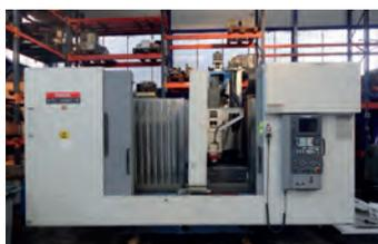
AV Centre vertical MAZAK VTC 300C
