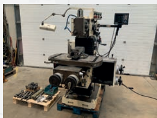
Fraiseuse universelle MAHO MH700 Courses X 500 mm - Y 300 mm Z 400 mm - Broche SA40 Table 820 x 480 mm Visu 3 axes FAGOR
